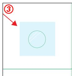
③ Window back gluing with PLA or cellulose film.
